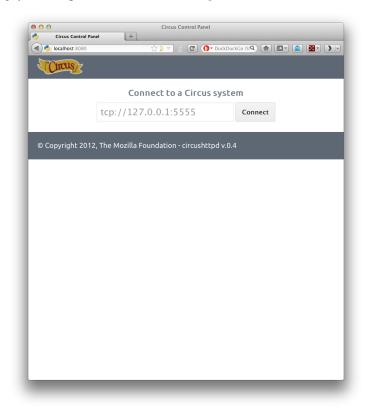
The Web Console is ready to be connected to a Circus system, given its **endpoint**. By default the endpoint is *tcp://127.0.0.1:5555*.
