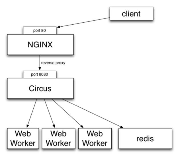
So, like Gunicorn, Circus is able to bind a socket that will be proxied by Nginx. Circus doesn't deal with the requests but simply binds the socket. It's then up to a web worker process to accept connections on the socket and do the work.
